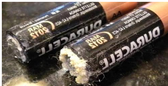
Figure1: leakage in chemical batteries
